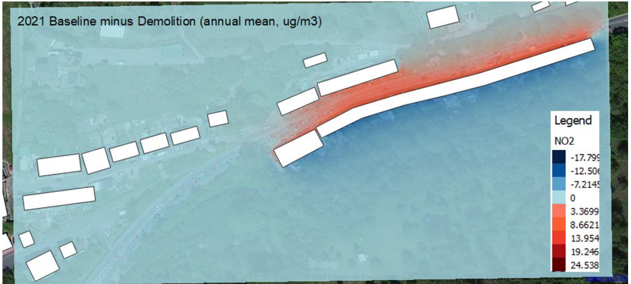
Figure 4-16 NO 2 difference plot for 2021 Scenario 3 (red areas = lower NO 2 concentrations, blue = higher)
